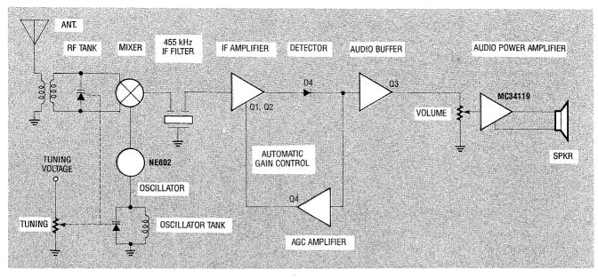
FIG. 1—BASIC BLOCK DIAGRAM of our superhet shortwave receiver. It's a true superheterodyne designed to tune 8.5 to 11 MHz in two bands.
