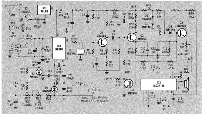
FIG. 2—SCHEMATIC FOR THE SHORTWAVE RECEIVER. The unit is powered from a 9-volt, battery, making it very portable. It's sensitivity of under a microvolt puts it in a class with some very high-performance receivers.
