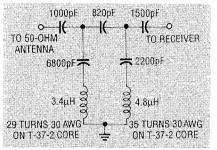
FIG. 3—THIS HIGH-PASS FILTER will attenuate AM stations by 40 dB. Its low-frequency cutoff is about 2.2 MHz.
