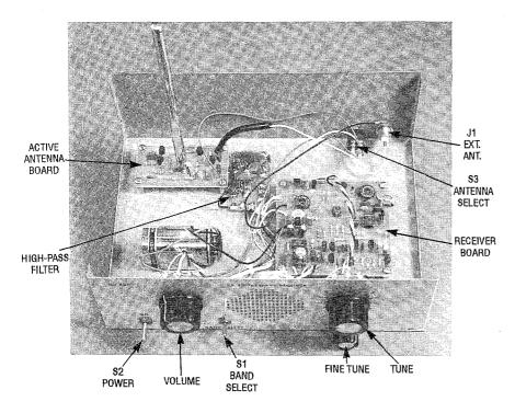
FIG. 5—THE INSIDE OF THE PROTOTYPE RECEIVER. Note that the active antenna and the 2.2-MHz high-pass filter are used in the prototype, although they are not mandatory.
